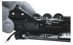
MAKE NOTE OF THE ECCENTRIC CRANKS IN REALTION TON THE AXLE IF THE DRIVER BEING CHANGED. THE ECCENTRICS MUST BE RE-ASSEMBLED IN THE SOME POSITION.
