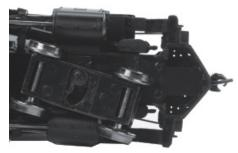
Engine Coupler Installed Underside View
