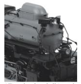
Gently remove the folded clamshell from the top of the smoke stack
