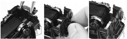
Lift Out Cover Plate & Pull Coupler Mechanism Out Through Pilot Hole
