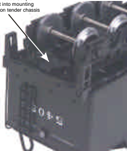
Install Kadee Coupler Mount into mounting holes on tender chassis
