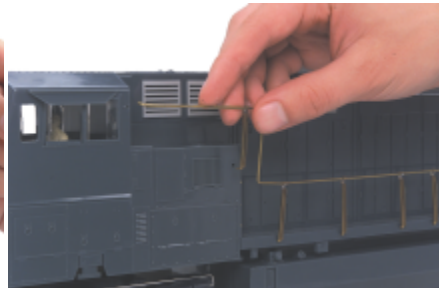
Figure 16: Handrail Separation From Cab
