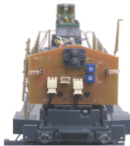
Figure 21: Front Locomotive Light Location
