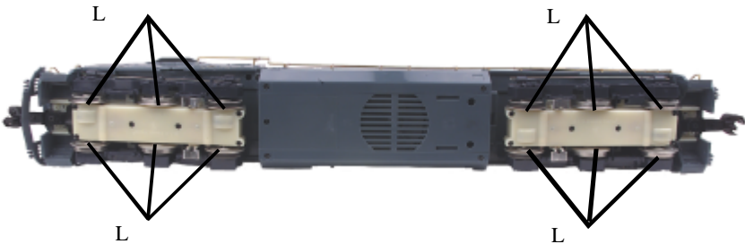
Figure 10: Lubricating The Chassis
