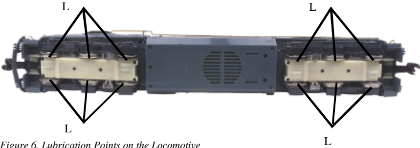
Figure 6. Lubrication Points on the Locomotive
