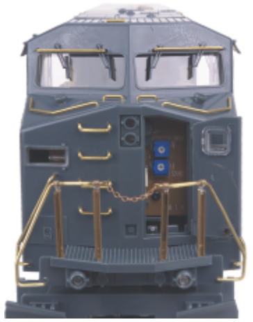
Figure 9: Manual Volume Adjustment (lower knob)
