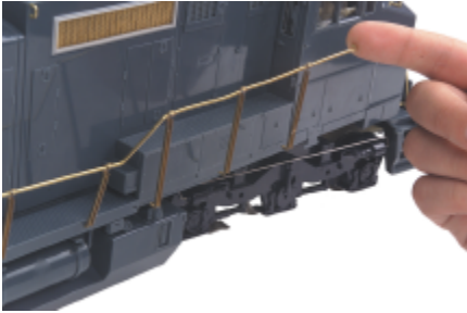
Figure 15: Handrail Separation From Cab
