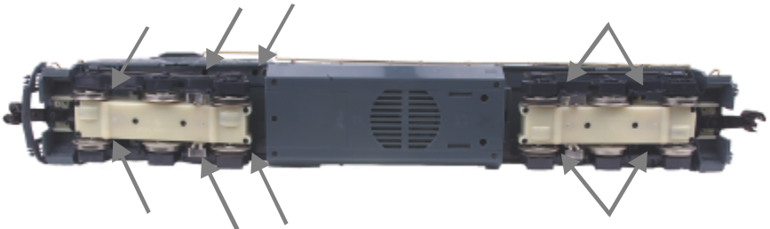
Figure 14: Body Mounting Screw Locations
