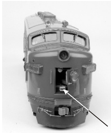
Figure 28: Battery Recharging Port
