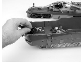
Figure 25: Pulling the lights out of the guides.
