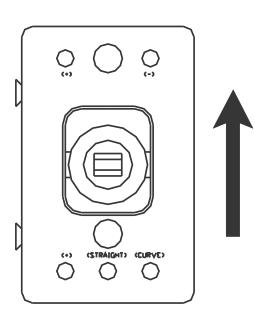
Push the remote switch lever toward the transformer lead wires to align the switch points to the curved direction.
