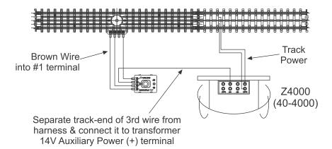
3. Auxiliary Power Operation: (Auxiliary Power not from same transformer as Track Power):
