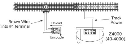
2. Auxiliary Power Operation: (Auxiliary Power from same transformer as Track Power):
