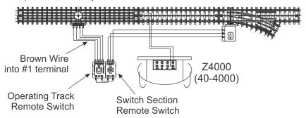
5. ScaleTrax<sup>™</sup> Operating Track Section & Switch wiring -Auxiliary Power Operation (recommended for Digital Command System (DCS) operation):
