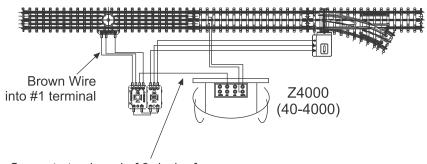
Separate track-end of 3rd wire from harness & connect it to transformer 14V Auxiliary Power (+) terminal
