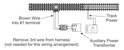
4. ScaleTrax<sup>™</sup> Operating Track Section & Switch wiring - Track Power Operation (not recommended for Digital Command System (DCS) operation):
