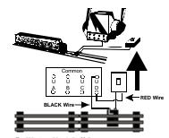
Figure 7: Wiring Up A Bell Button
