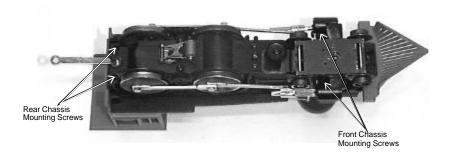
Figure 10: Removing The Boiler From The Chassis
