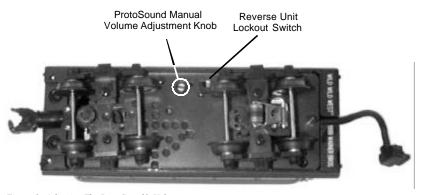
Figure 6: Adjusting The ProtoSound® Volume
