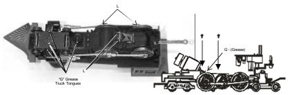
Figure 8: Lubricating The Locomotive Chassis
