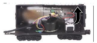
Figure 9. Replacing the Battery
