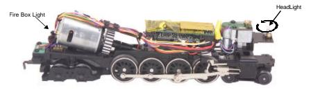
Figure 8. Replacing the Headlight and the Fire Box Light
