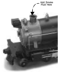
Figure 4. Add Smoke Fluid Through the Smoke Stack
