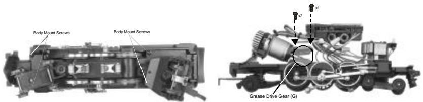
Figure 3. Locations of Body Mount Screws and Diagram for Greasing the Drive Gear
