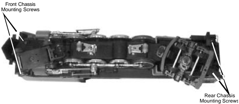
Figure 10: Removing The Boiler From The Chassis
