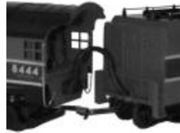
Figure 1: Plugging in the tender harness
