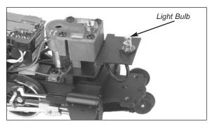
Figure 7 - Replacing the Headlight
