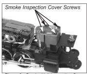
Figure 6 - Smoke Unit Inspection Cover
