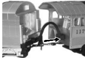
Figure 1: Plugging in the tender harness
