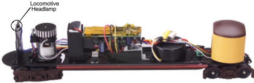
Figure 6a. Location of the headlamp in the Engine.
