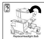
Oncethelocomotiveboilerhasbeenremovedfromitschassis, locate thebulbbracketasseenintheillustrationontherightand rotatetheheadlightbulbcounter-clockwisetoremove.
