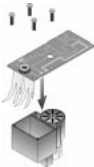
Figure 21: Servicing the Smoke Unit.
