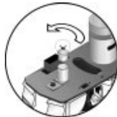
Figure 15: Removing the locomotive headlight bulb.
