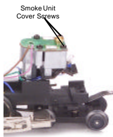
Figure 12. Inspection Cover Screws
