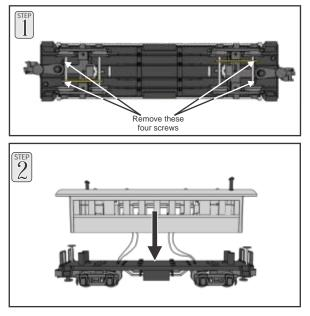
1) To remove the shell from chassis remove the four screws located underneath the trucks.
