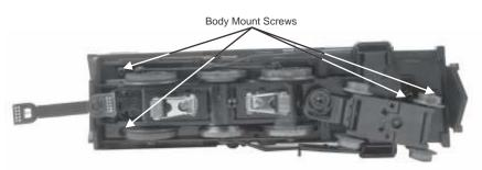
1. Remove the 4 body mount screws, locate the smoke unit assemby.
