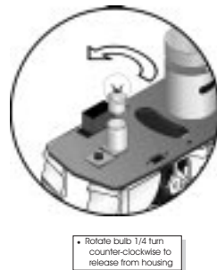
Figure 17: Removing the locomotive headlight bulb.
