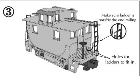
Step 3. Re-assembly is the reverse procedure of removal. Be careful when refitting the shell that you line up the ladders with the holes on the outside of the railings and insert the ladders into these holes before screwing the shell back to the chassis. Failure to line the ladders up correctly may cause damage to the ladders or the railings.
