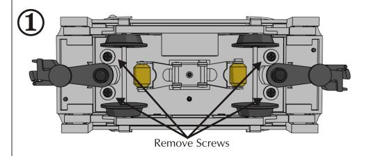
Step 1. Remove the four screws located underneath the caboose.
