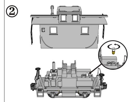
Step 2. Lift the shell off the chassis. Unscrew the bulb from its socket by turning it counter-clockwise.
