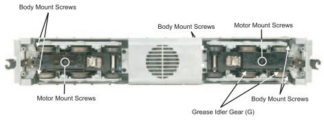
Figure 5. Body Removal Screw Locations
