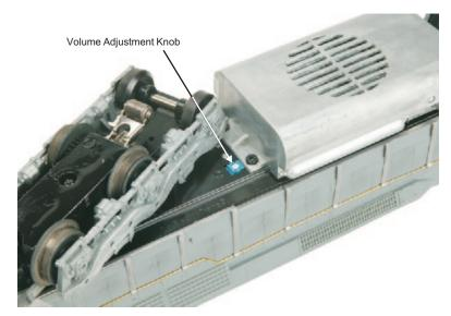
Figure 4. Manual Volume Adjustment Knob
