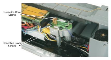
Figure 9. Inspecting the Smoke Unit Wick
