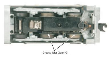
Figure 6. Greasing The Idler Gears
