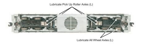
Figure 1. Lubrication Points on the Locomotive
