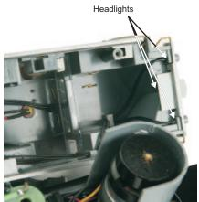
Figure 7. Replacing the Light Bulbs
