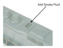
Figure 8. Filling The Smoke Unit
