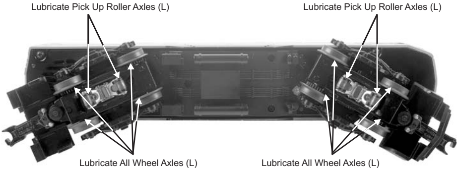
Figure: Lubrication Points on the Locomotive
