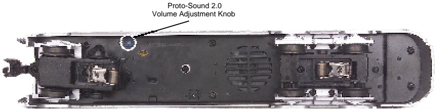
Figure 2: Manual Proto-Sound 2.0 Volume Adjustment
