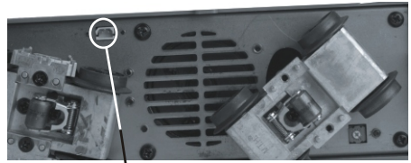
Battery Charger Port
