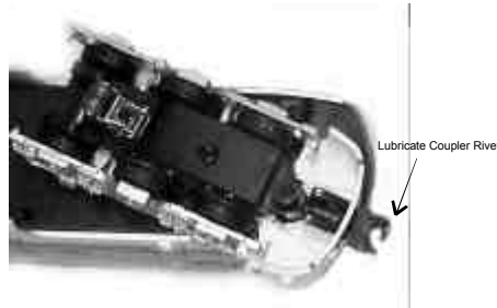
Figure 3: Lubricating The ProtoCouplers
