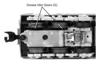
Figure 4. Greasing The Idler Gears
