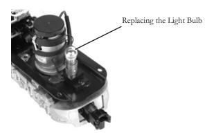
Figure 5. Replacing the Light Bulb
