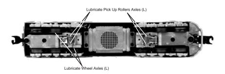
Figure 1. Lubrication Points on the Locomotive
