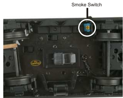
Figure 8: Smoke Unit Switch Location (Inside Tender Hatches)
