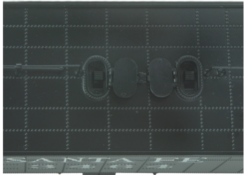
Figure 2: Selecting 2-rail or 3-rail power input setting
