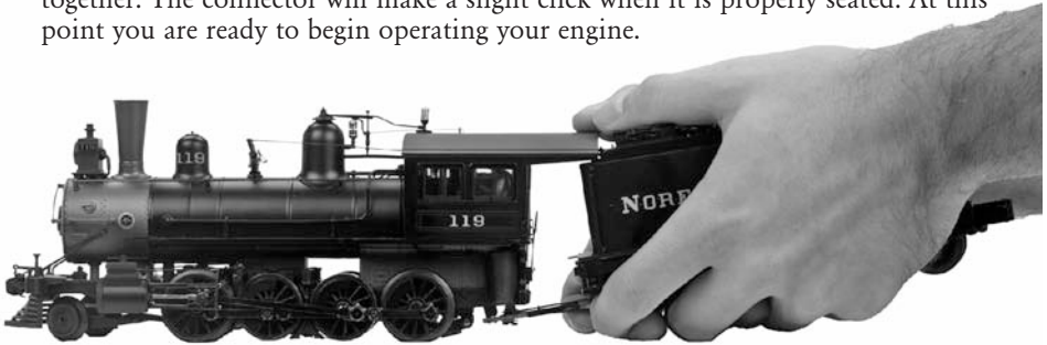
Figure 5: Connecting Locomotive to Tender
