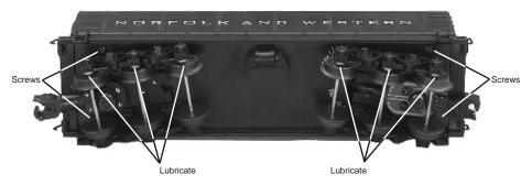
Figure 4. Lubricating the Chassis and Location of Body Mount Screws on Auxiliary Tender
