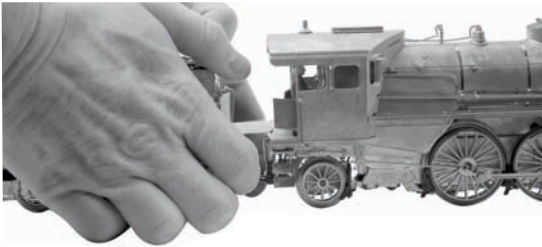
Fig. 10: Pushing Connectors Together
