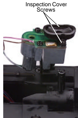
Figure 5. Inspecting the Smoke Unit
