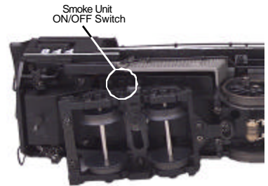
Figure 4. Smoke Unit ON/OFF Switch
