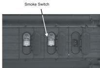
Figure 5. Smoke Unit Switch Location
