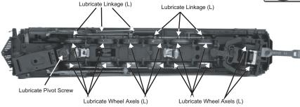
Figure 4. Lubrication Points on the Locomotive
