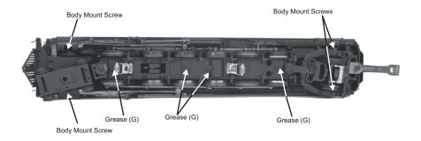
Figure 9. Removing the Body and Lubricating the Grease Points
