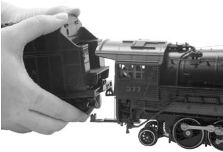
Figure 4: Connecting Locomotive to Tender
