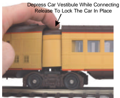
Figure 4: Connecting The Cars
