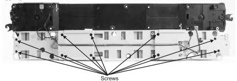
4. To replace the interior lights first remove the connector from the top of the interior then unscrew the light boards and remove and replace the entire assembly.
