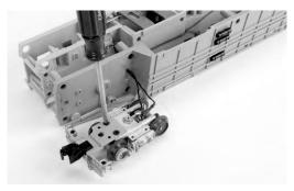
4. Attach the pilot to the bottom of the base. Then remove the coupler from the truck and reattach the truck to the base.
