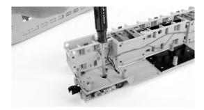
3. Remove the pilot from the truck by removing the 2 screws on top of the truck.
