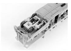
5. Line the spacer & Kadee Coupler up w/the holes in the undercarriage and screw them down.
