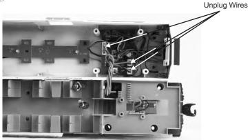
4. To replace the interior lights unscrew the light boards and unplug the wire connector. Then remove and replace the entire assembly.
