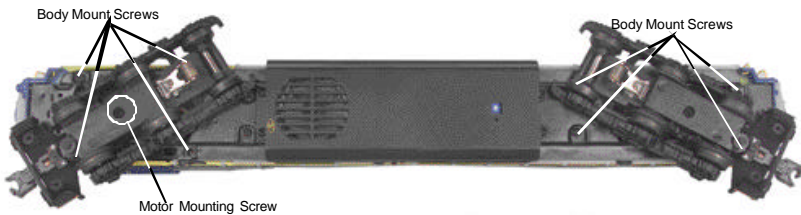
Figure 5: Body Removal Screw Locations
