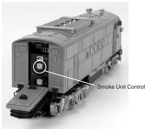
Smoke Unit Control
