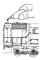
Figure 3: Filling The Smoke Unit
