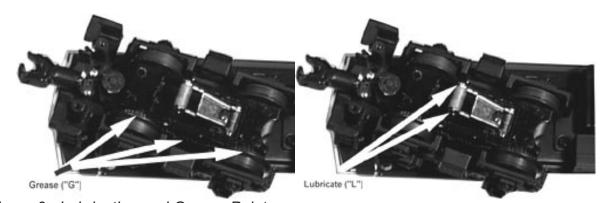
Figure 9: Lubrication and Grease Points
