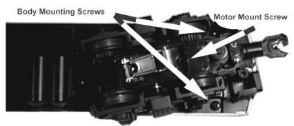
Figure 8: Removing The Body From The Chassis
