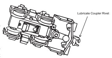
Figure 5: Lubricating The Proto-Coupler™
