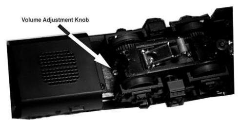
Figure 6: Manually Adjusting The ProtoSound Volume
