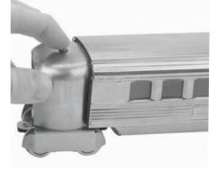
Figure 4: Step 4 [Locking Vestibule in Place]
