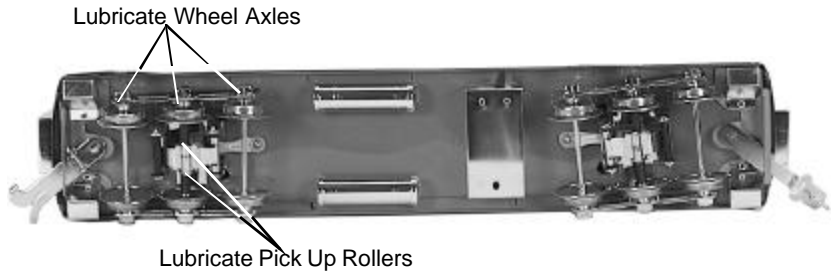
Fig. 3 Lubricating the Passenger Car
