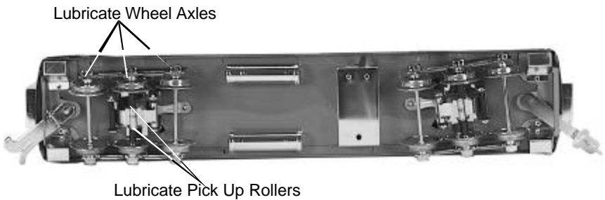
Fig. 3 Lubricating the Passenger Car
