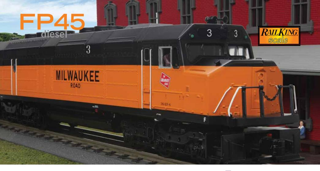
Designed in 1967 at the request of the Santa Fe, the FP45 was basically an SDP45 road switcher with a streamlined cab unit body. The "P" in FP45 indicated a passenger diesel with a steam generator for train heat. Having a sleeker, more aerodynamic look than a road switcher, the FP45 blended better with its passenger consists; the fully enclosed body also reduced wind resistance and allowed the crew to perform troubleshooting and minor maintenance on the road.
