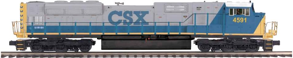
In the horsepower race of the 1990s - which turned out to be a passing fad — the Holy Grail became a 6000 hp diesel. But neither EMD nor GE had a prime mover capable of being upgraded to that size. As a stopgap measure, EMD added four cylinders to its proven model 710 engine to create the 5000 hp, 20 cylinder, 80 foot long SD80MAC in 1995. Conrail was the only taker, rostering all 30 units produced and later passing them on to successor CSX.
