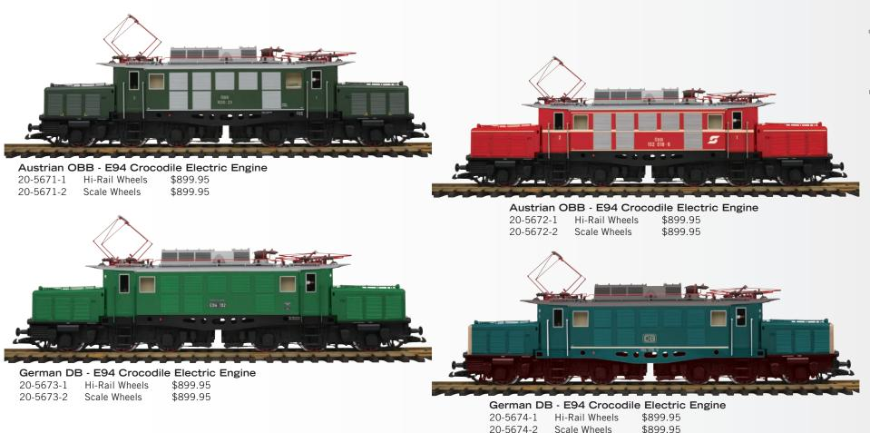
Whether referred to as an E94 or BR 194 or Iron Pig, the German bred E94 electric freight locomotive was developed to tackle the steep grades of Southern Germany just as the more famous Swiss Crocodiles were created to combat the Gotthard line in Switzerland. Equipped with just six axles, weighing over 120 tons and measuring nearly 19 meters in length, the "German Alligator" could haul a 1,000 ton train up a 1.6% grade.
