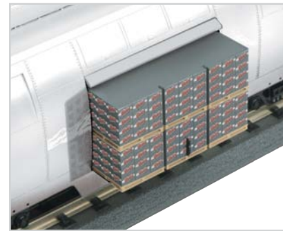
Load Slides Out For Smoke Fill Up
